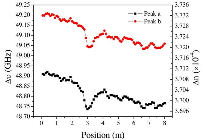
Fig. 5. (Color online) Measured distributed birefringence of 8 m panda fiber using peaks a and b.
