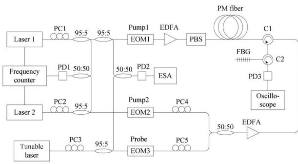
Fig. 1. Experimental setup: PC, polarization controller; EOM, electro-optic modulator; PBS, polarization beam splitter; C, circulator; PD, photo-detector; EDFA, erbium-doped fiber amplifier; ESA, electrical spectrum analyzer; FBG, fiber Bragg grating.
