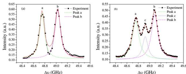
Fig. 4. (Color online) Typical TBG spectra in panda fiber: (a) two- and (b) three-peak spectra.
