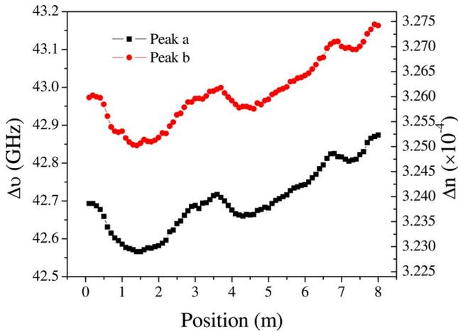
Fig. 3. (Color online) Measured distributed birefringence of 8 m bow-tie fiber using peaks a and b.
