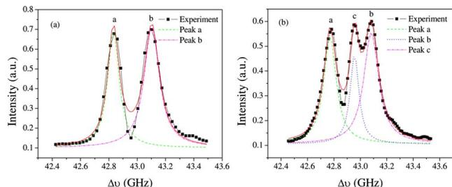
Fig. 2. (Color online) Typical TBG spectra in bow-tie fiber: (a) two- and (b) three-peak spectra.
