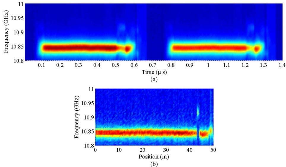
Fig. 4. Measured 3-D BGS of the sensing fiber (a) with 52/50 ns differential double-pulse and (b) after differential process. An 80-cm section of fiber located at the position of  $\sim 44$  m was stretched.
