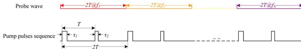
Fig. 2. Scheme of the probe wave and the pump pulses sequence for a high-spatial-resolution F-BOTDA. The frequency of probe wave is scanned from  $f_1$  to  $f_N$ , and for each frequency its duration is  $2T$ . The pump pulses sequence includes many pairs of differential double-pulse, where the interval between the them also equals  $2T$ .
