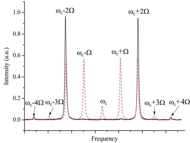
Fig. 1. Measured optical spectra of the modulated light. The solid curve shows the second-order sidebands dominating the spectrum when the modulator operates at the maximum transmission point and  $\gamma = 2.405$ ; the dashed curve shows a complex spectrum with more frequencies when the modulator operates deviating from the optimal condition.
